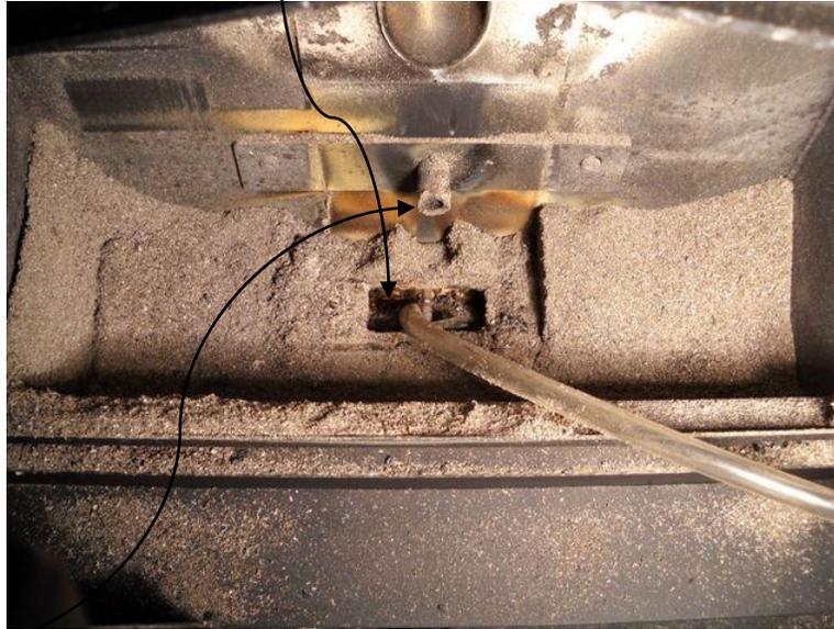
Clean the area around the igniter tube and carefully clean the end of the igniter of any buildup.
